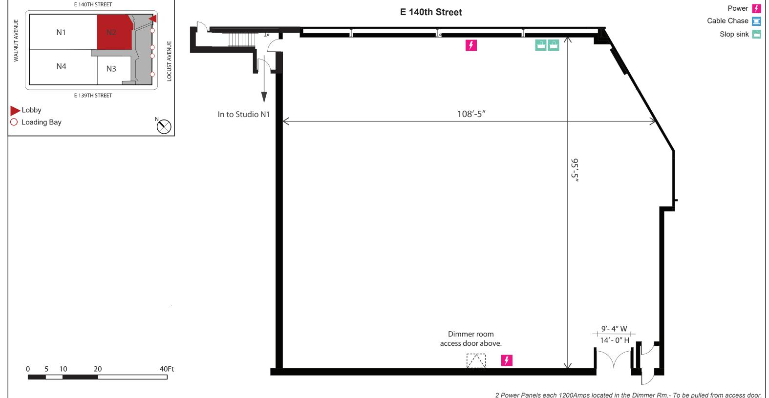
2 Power Panels each 1200Amps located in the Dimmer Rm.- To be pulled from access door.
